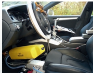
Proving Ground Driving System SfpHybrid
